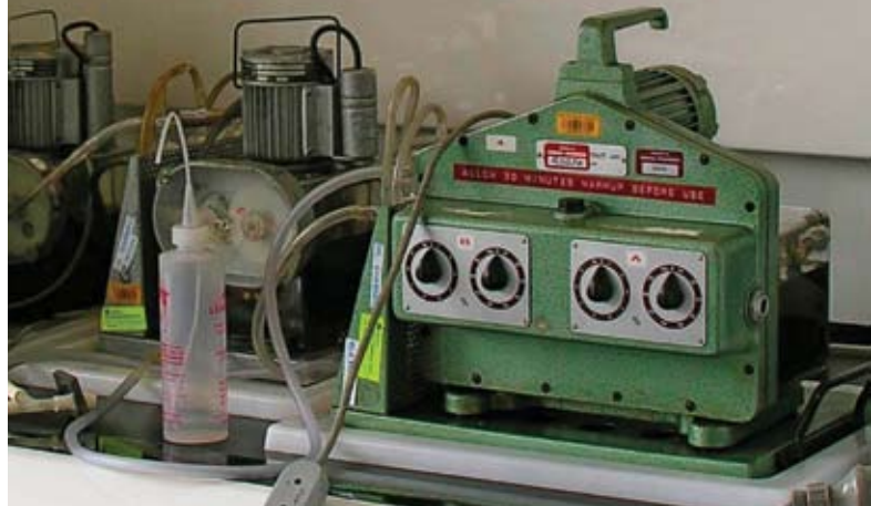
Wosthoff precision gas mixing pumps used to prepare standard test gases at the Mine Safety Technology Centre.
