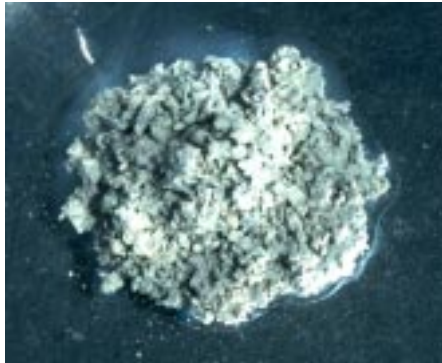
Dispersion score 1: Slight dispersion recognised by slight milkiness of water adjacent to aggregate
