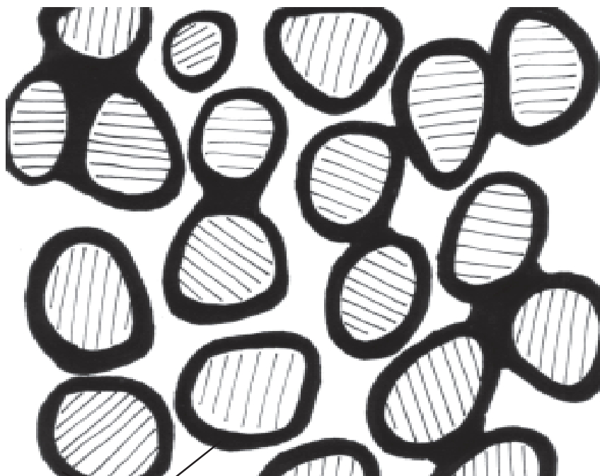
Figure D9-4. Soil at field capacity (good balance of water and air)
