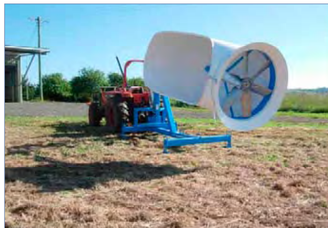
Frost Stoppa with large propeller and fibreglass housing.
