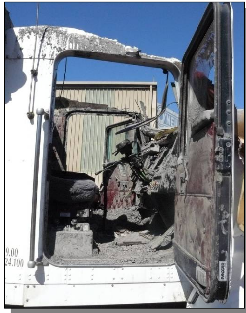
Driver's side view of the Kenworth T401 truck cabin showing the damage caused as a result of the incident
