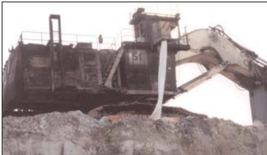
The safety chute hanging from the burnt-out excavator at Bulga Coal
