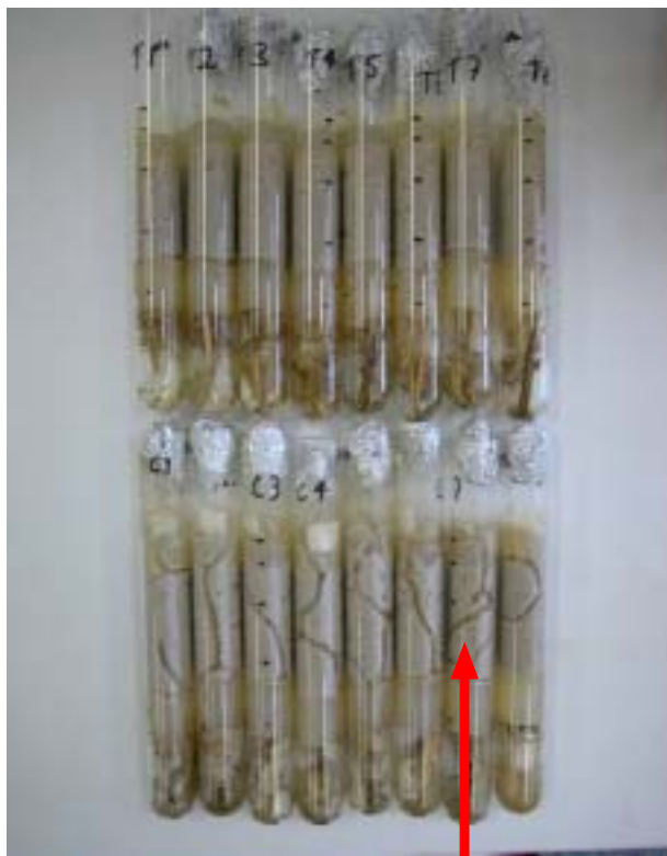
Above: Termite barrier trial (note tunnelling) Top - Barrier mixed with extract Bottom - Barrier untreated (control)
