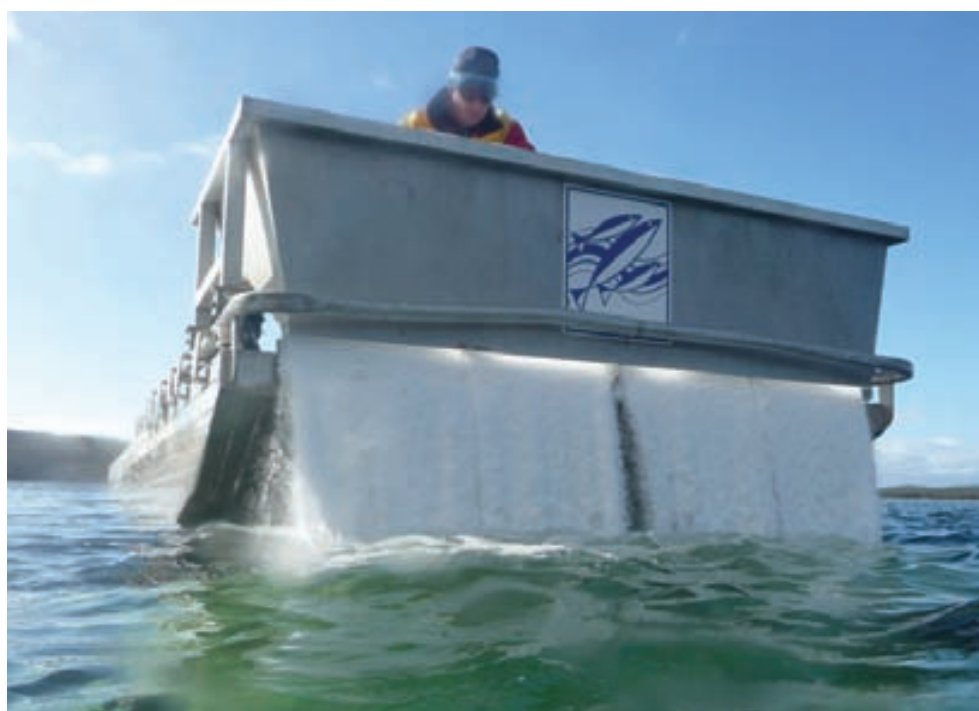
Applying salt at Wallagoot Lake for Caulerpa control using I&I NSW purpose-built punt. Photograph James Sakker I&I NSW
