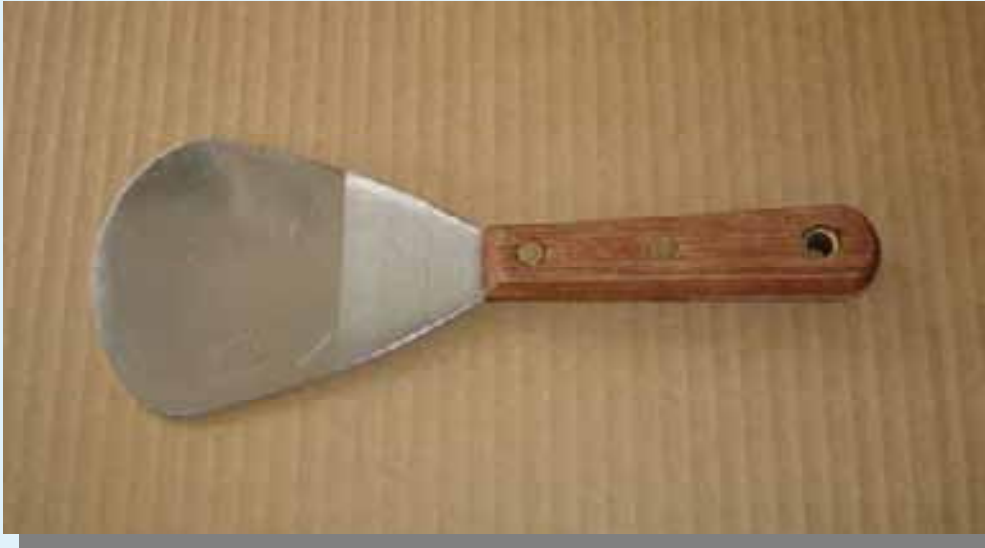
Figure 14 A metal paint scraper with its corners and sharp edges ground off to minimise injury to broodstock being collected from the wild
