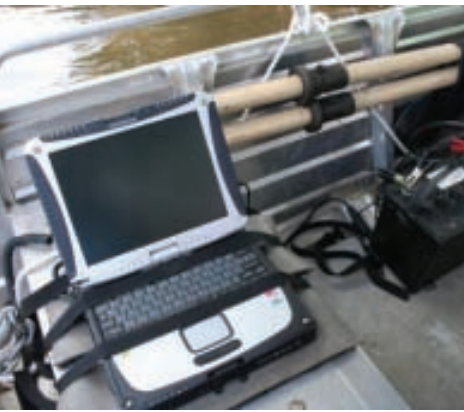
Panasonic Toughbook® laptop with built in GPS and GIS software. Photo: Brian Worboys
