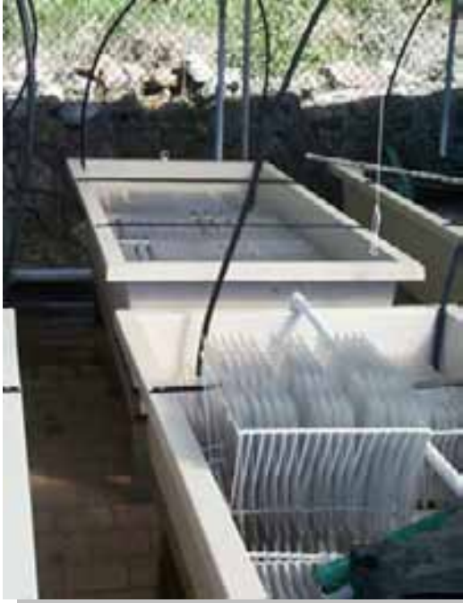
Figure 33 Standard 600 x 300 x 1.5 mm clear PVC nursery settlement plates. These plates are mounted on their long edge in plastic coated or stainless steel wire baskets that hold 14 to 18 plates.
