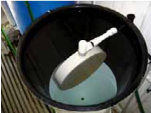
Figure 29 Overhead view of incubation/larval rearing vessel showing the internal surfaces that must be smooth and scratch-resistant, and the base, that should be conical and white to aid hygiene and visual assessment of the condition of developing larvae.
