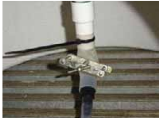
Figure 30 A thumb-screw clamp attached to a clear silicon-rubber air input and drainage hose is the simplest way to provide regulated slug air-flow within larval rearing vessels.
