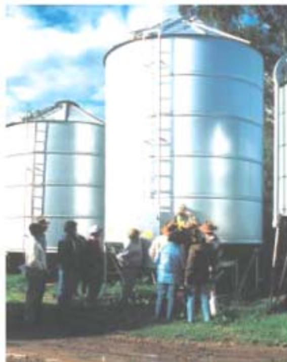
Riverina Organic Farmers Organisation members inspect a grain silo with CO 2 disinfestation capability.
