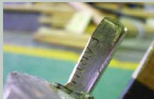
SB11-03 A 3 pin plug with the earth pin filed down to enable use in a 10A socket outlet
