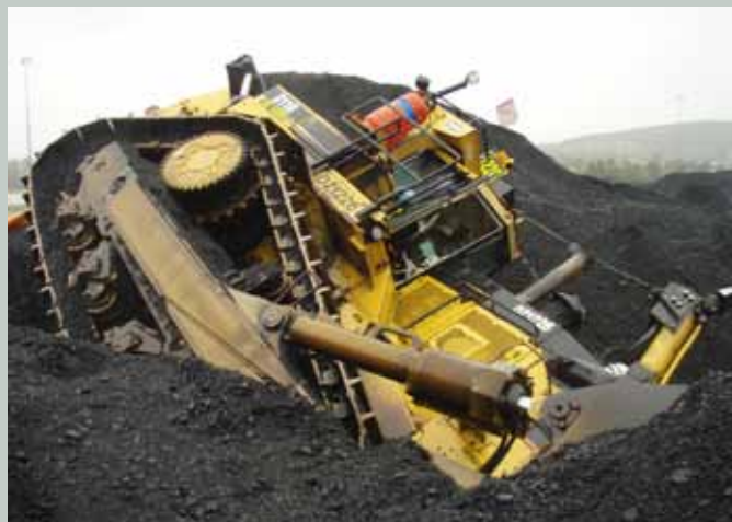
SA11-09 Stockpile dozer lodged in reclaim valve
