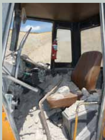
SA11-03 Material from a stockpile collapse partly filling a loader cabin
