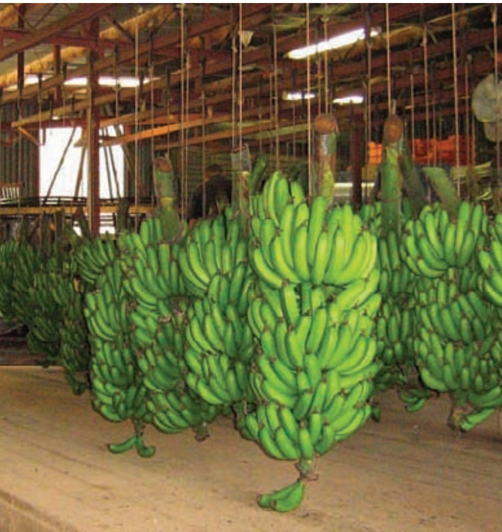
Bunches hanging on butcher rails ready for dehanding onto a packing wheel.
