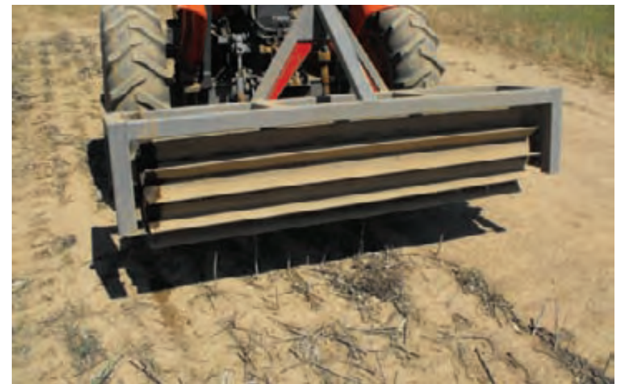
A crimp roller can reduce the need to cultivate for weed control.
