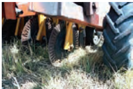
A coulters, tine and press wheel mechanism for direct drilling seed minimises soil disturbance.
