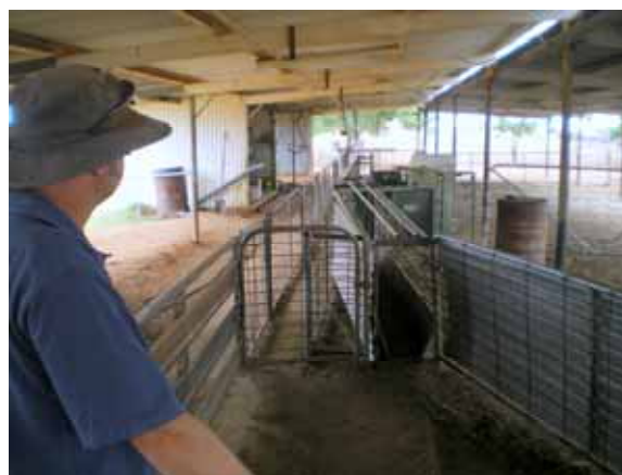
Figure 1. A drafting system incorporating a simple set of scales that use radio frequency identification (RFID) and a computer to provide a wide range of sheep management information.
