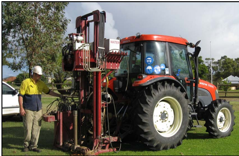
Tractor-mounted sonic drill rig used for extracting soil cores
