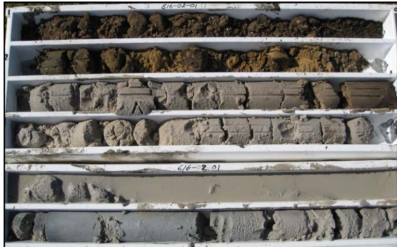
A 6m soil core extracted from a site using sonic drilling.
