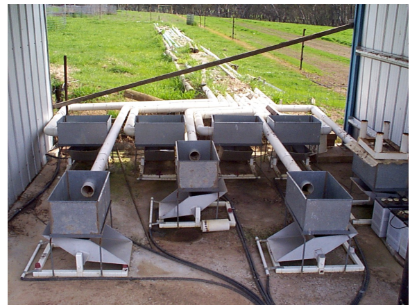
Tipping buckets for water runoff measurements
