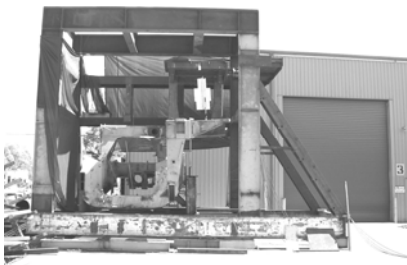
Destructive Testing Caterpillar 793 Dump Truck O/Fit ROPS
