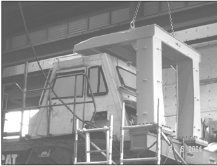
Installation of the Overfit ROPS Caterpillar 793 Dump Truck
