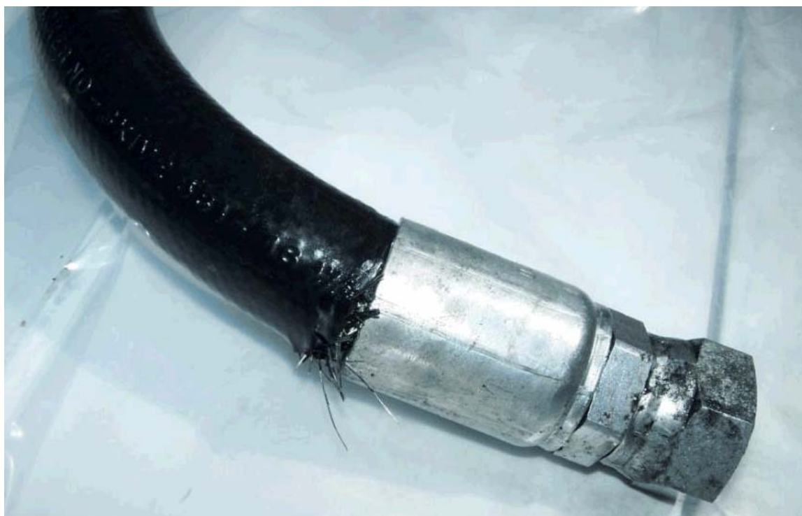
Figure 1 – Failed hose showing failure adjacent to ferrule
