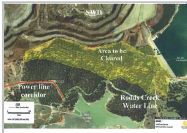
This diagram shows the area cleared in May 2008 below the South Waste Dump and Rodds Creek Dam.
