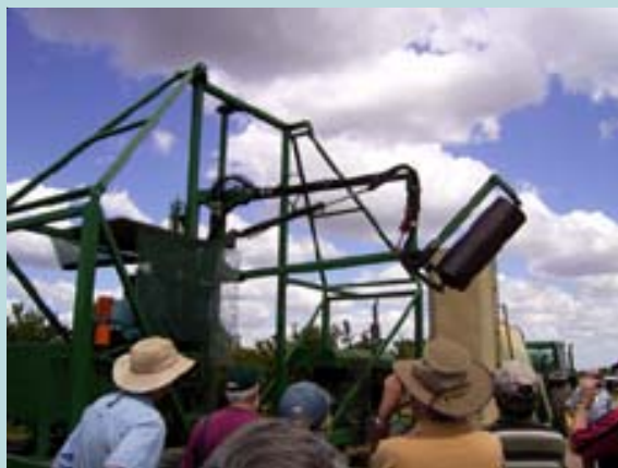
This thinning machine is used to remove sunburnt fruit on the tops of mandarins at McLennans orchard.
