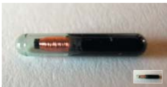
Fig. 10.2 PIT tag that is inserted under the skin of fish, actual size is 11mm x 2mm.
