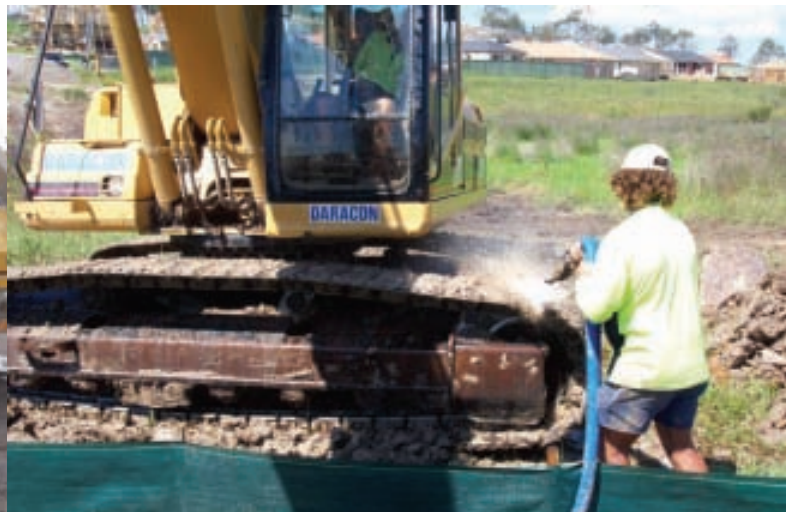
Tracks and track frames must be cleaned thoroughly. Photo: Brian Worboys
