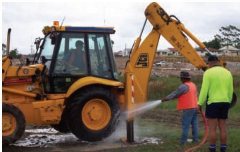
Thoroughly clean tyres and rims of wheeled tractors. Photo: Brian Worboys
