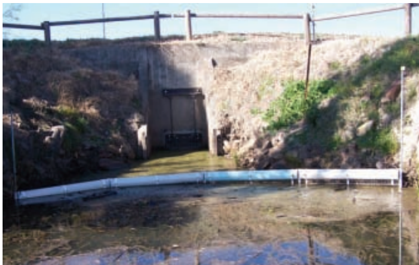
PVC and mesh boom commercially designed to contain alligator weed fragments. Photo: Graham Prichard
