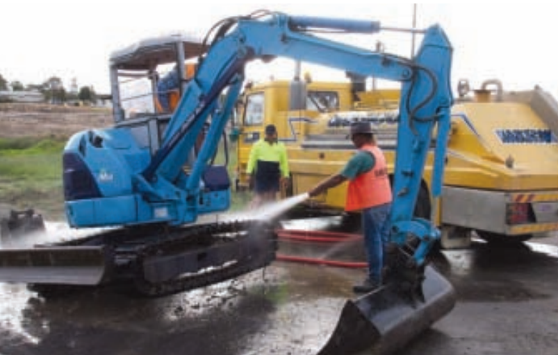
The arm of the excavator may be used to lift each track off the ground. Photo: Brian Worboys
