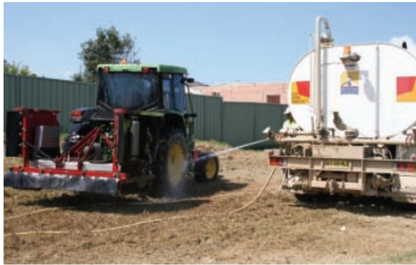
Water tankers can be used for onsite washdown. Photo: Brian Worboys
