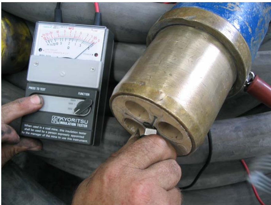
Figure 22: Earth continuity test from phase barrier to plug body for a typical 300 Amp restrained plug
