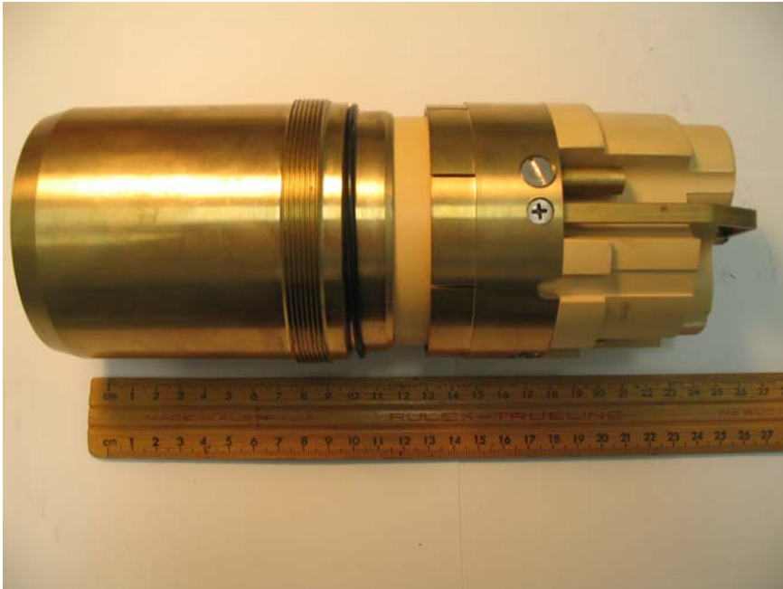
Figure 17: Front view of the disassembled Minto Industrial Products 300 Amp Restrained Plug
