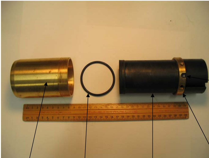
Figure 11: Stripped down view of the Macey 150 Amp Restrained Plug
