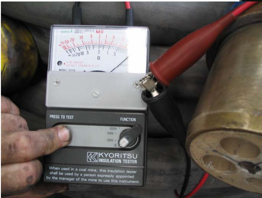
Figures 20: Zero check for Ohmmeter
