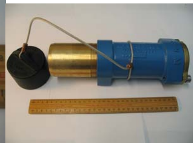
Figures 7 and 8: Crouse Hinds (Macey) 150 Amp Restrained Plug
