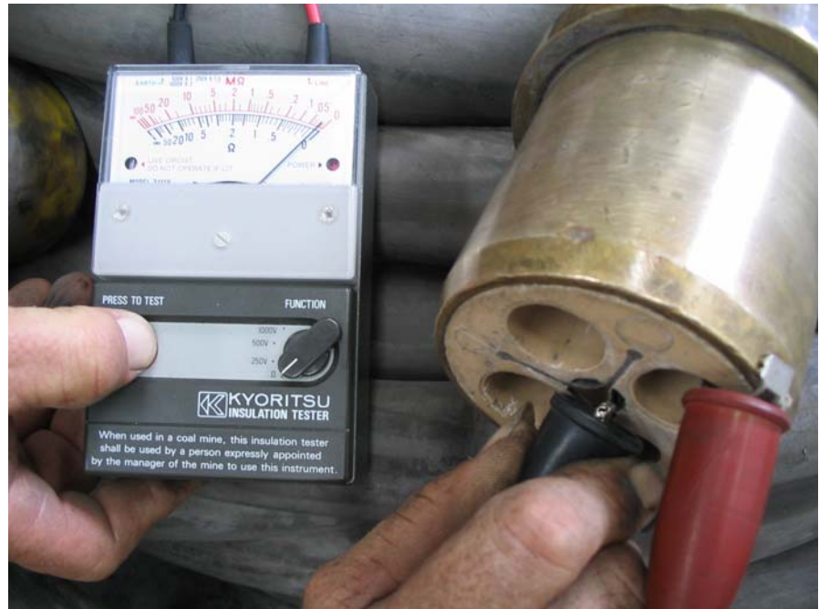
Figure 21: Earth continuity test from phase barrier to nose-cone for a typical 300 Amp restrained plug
