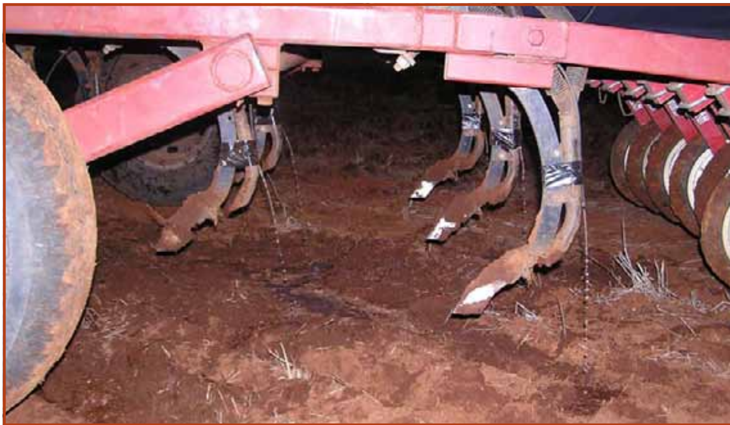
Seeder liquid injection setup at used to apply liquid micro-nutrient treatments at sowing.
