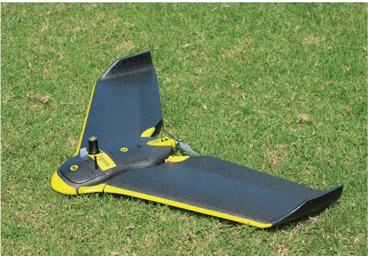
Figure 1. Drone type EBEE RTK ready for take off.
