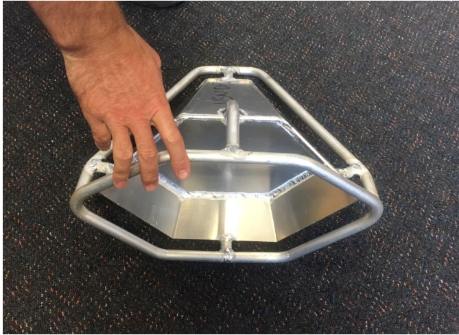
Photo: The Fish-eye BRD is a behavioural-type BRD that may be used.
