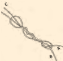
5. Moisten the line and form a knot by pulling tag A against loop C.
