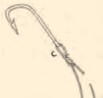
8. The loop C disappears as the knot slides down on to the eye.
