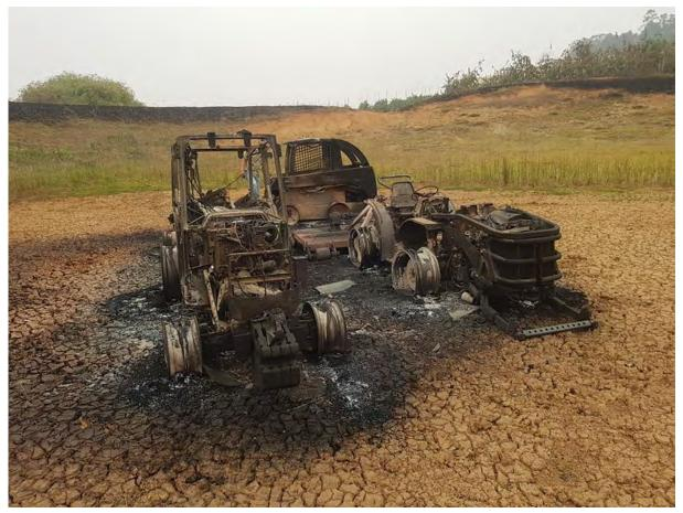
Figure 30. Despite being placed in the centre of a dry dam, this orchard machinery was lost due to the intense fire and ember attack.
