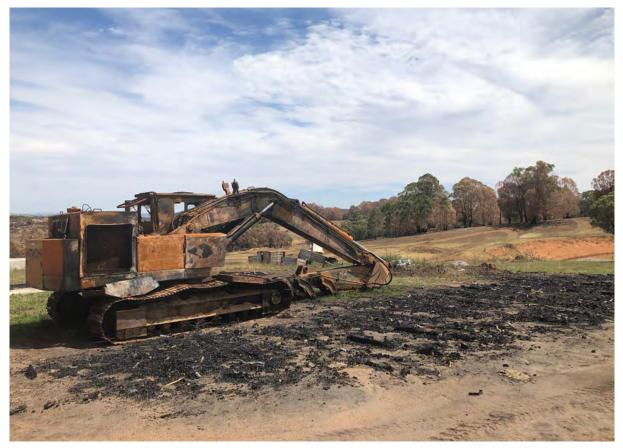
Figure 31. This excavator was parked in an open area but unfortunately was adjacent to a stack of timber harvest bins.
