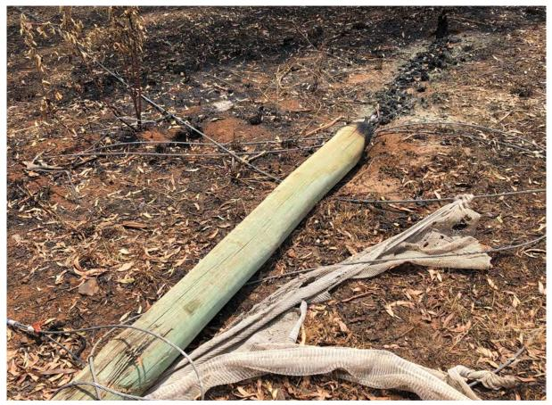
Figure 25. Chemical ash residues from burnt treated pine poles presented a risk to stock and human health and required careful management.
