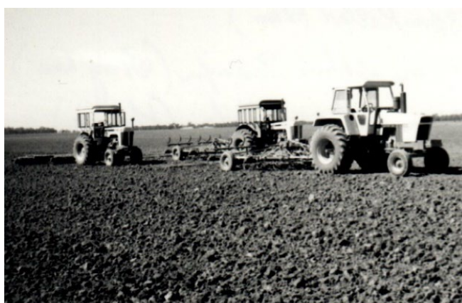
Figure 2. Traditionally preparing stubbles in 1972 prior to changing to stubble retention and direct drilling. Tractors from left are Case 830 towing a Furphy spike roller; Case 930 towing a 21-tine Shearer scarifier; and a Case 970 towing a 25-tine Shearer scarifier. (Photo: Ian Lea)
