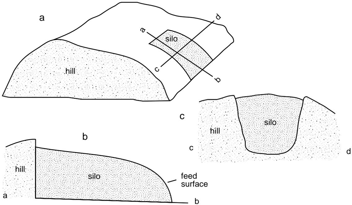
**Figure 4.6. Building silage storage into a hill is the preferred method of in-ground storage for any silage. Pits built below ground level are more risky.**
