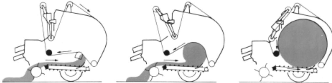
**Figure 3.2. Bale formation in fixed-chamber balers. The baler on the left uses belts; the one on the right uses rollers.**
