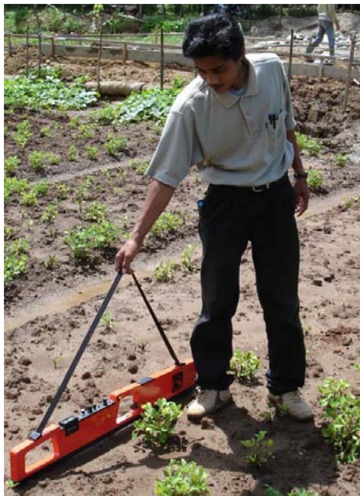
Fig. 1. The electromagnetic induction instrument (EM38) is used to assess salinity level in the tsunami-affected areas of NAD province, Indonesia.
