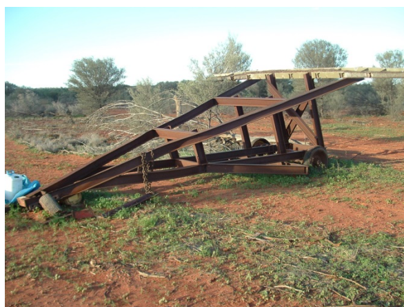
Figure 4. Trailing implement designed to take the tops out of the trees, leaving smaller lateral branches and the base of the tree intact.
