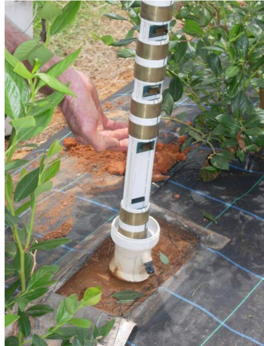
Figure 3 EnviroSCAN showing electronic sensors at various depths
