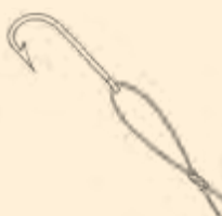
7. This forms a slipping knot and loop.
