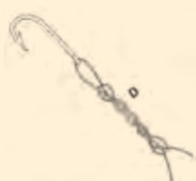
6. As you continue to pull on the tag all of the spirals in the tag are transferred to the loop D.
