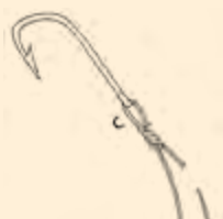
8. The loop C disappears as the knot slides down on to the eye.
