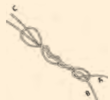
5. Moisten the line and form a knot by pulling tag A against loop C.
