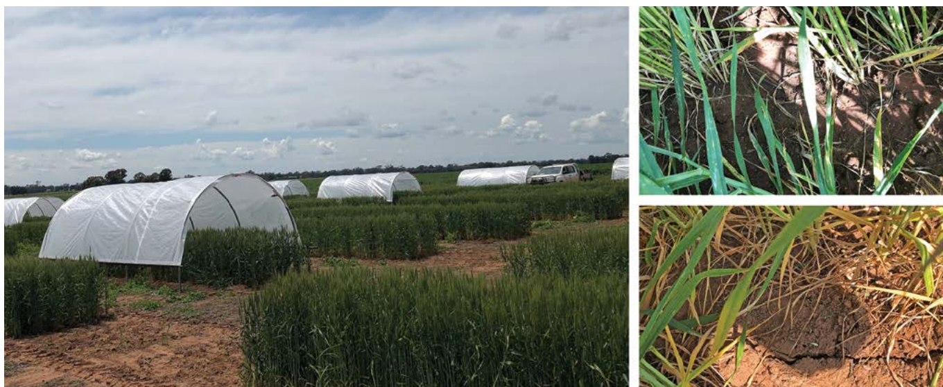
Figure 1 Portable rainout shelters covering wheat plots to exclude rainwater at Tootool, southern NSW. Photos taken at anthesis showing wetter surface soil in the rain-fed plot (top right) compared to the plot with rainout shelter (bottom right).
