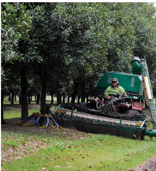
A sweeper moves less soil than a blower, but can create a depression along the drip line that might need management.
