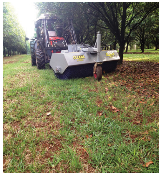
Road brooms are a recent innovation in macadamias. They leave living ground cover relatively undisturbed.
