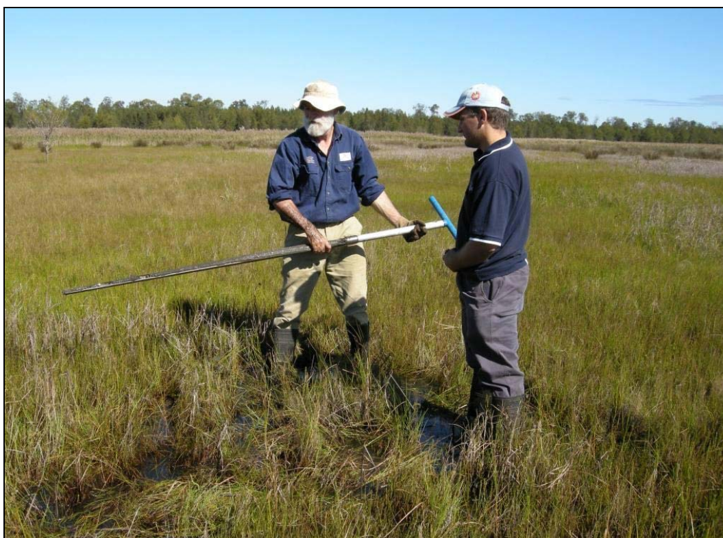
Figure 37: Soil core sampling at Tomago site T6 (photo: J Fredrickson)
