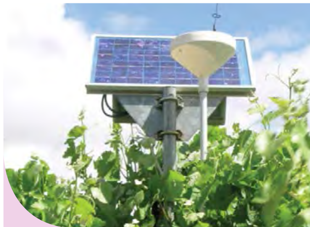
Figure 4: Automatic weather stations (AWS) monitor the vine canopy for leafwetness, rainfall, relative humidity (RH) and temperature. These are critical to the life cycle of downy mildew. An AWS, like this Australian designed and built Model T MetStation ® , is also a disease predictor. It processes the weather data it records and signals infection events by a series of red lights if infection is active. This provides a disease risk statement on-site in the vineyard or it can be relayed directly to your home computer. This information is often critical to refining optimum spray timing in your vineyard.
