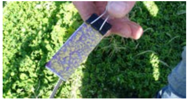
Figure 79. Water-sensitive paper after spraying. Photo: Adrian Englefield, NSW DPI.
