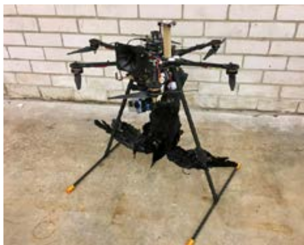
Figure 46. UAV equipped with horn tweeter and taxidermied crow.
