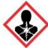
Severe Health Hazards
