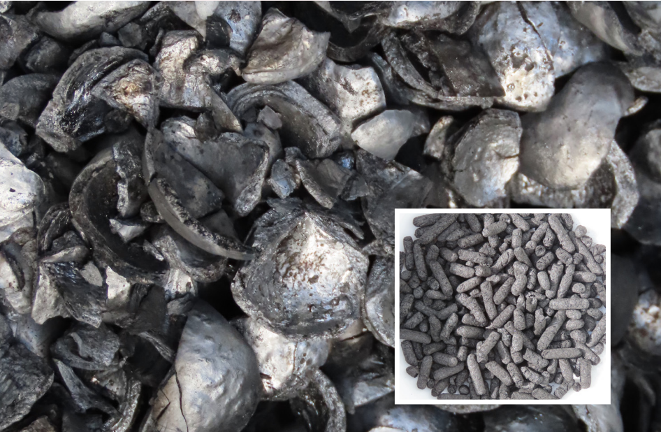
Above: Biochar made from macadamia shells and (inset) from pelletised canola stubble, a form ready for use.
