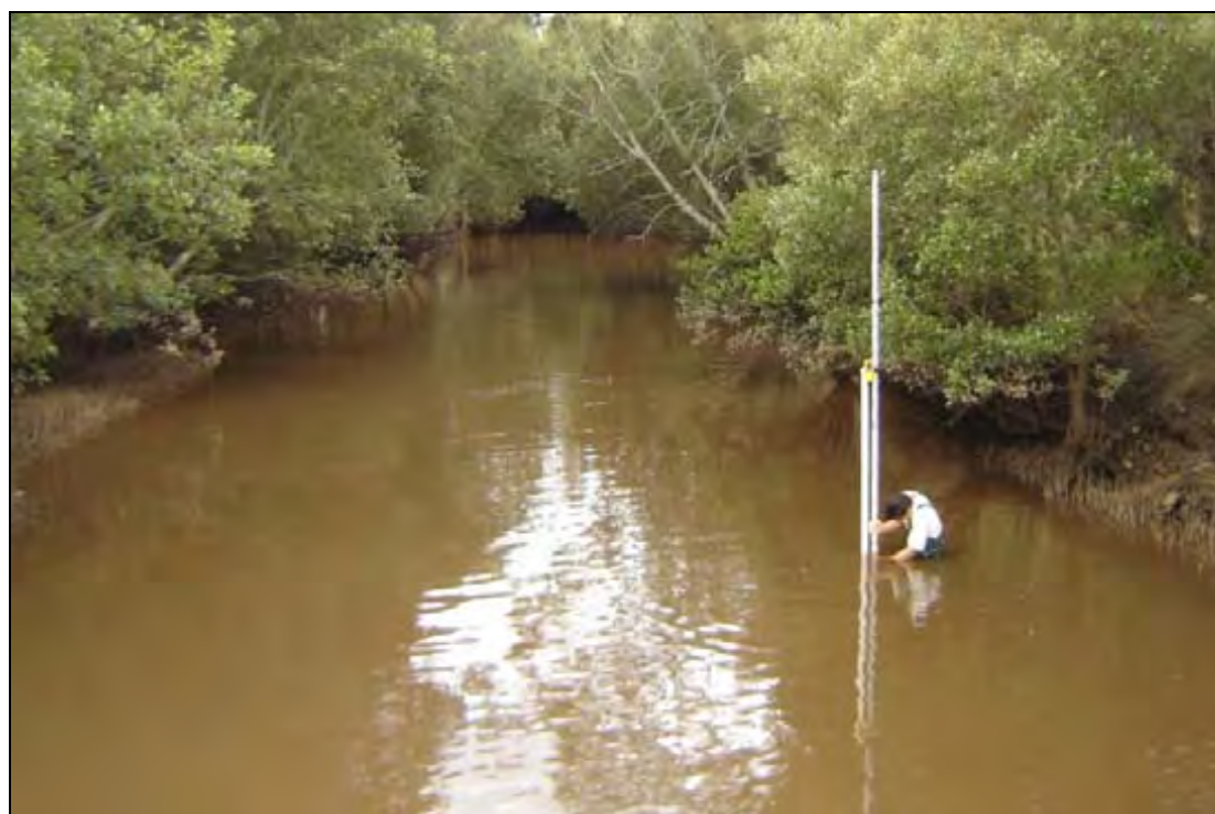
Figure 10 Water level probes were deployed upstream and downstream of the floodgates to record changes in water level with tide.
