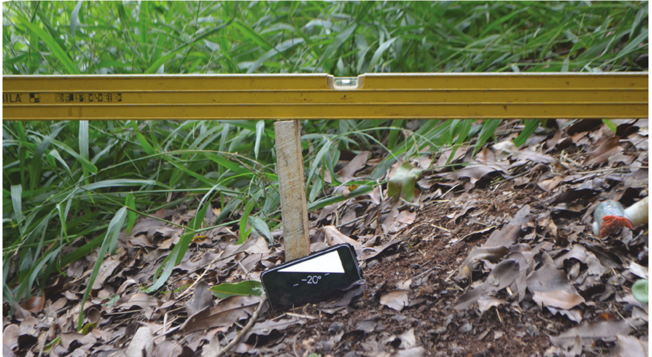
Figure 22. Measuring slope using a level and a smart phone.
