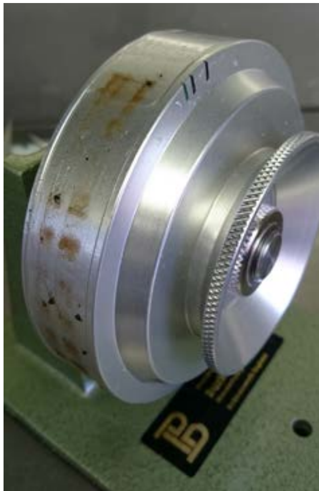
Figure 21. Exposed spore tape on the drum, used for trapping spores in vineyards.
