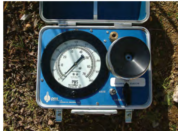
Figure 1. Example of a pressure chamber used to measure leaf water potential.
