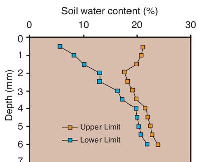
**Figure 2.** A graph of soil water content that shows that lucerne extracted approximately 310 mm of stored soil water from this profile. The difference between the upper limit and the lower limit equals the amount of water extracted.
