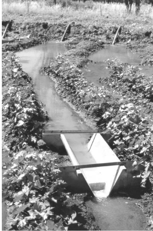
Figure 5. Measuring siphon flow using a flume
