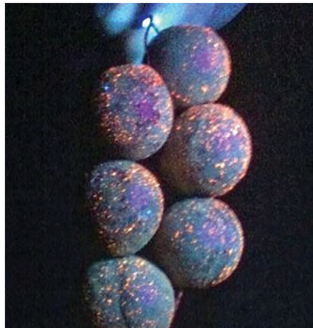
Figure 17. Using fluorescent dyes to demonstrate coverage. Photo: Jeremy Bright.
