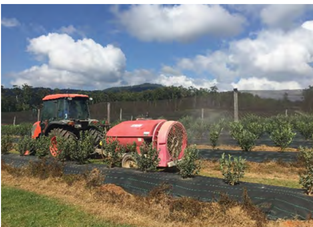
Figure 1. An axial air-blast sprayer. Photo: Melinda Simpson.
