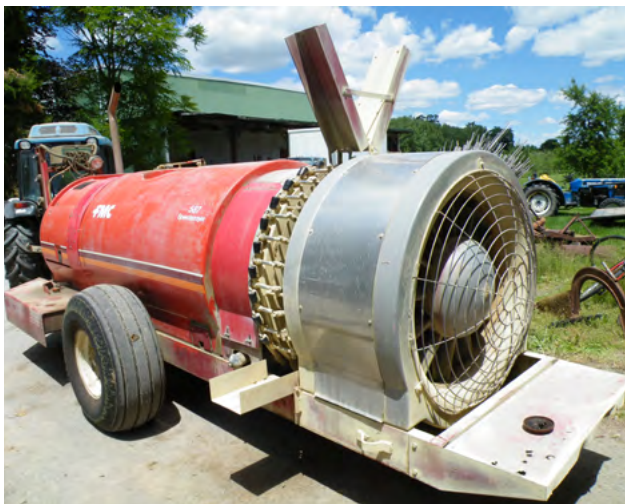
Figure 9. Deflectors on an air-blast sprayer. Photo: Jason Deveau, Sprayers 101.
