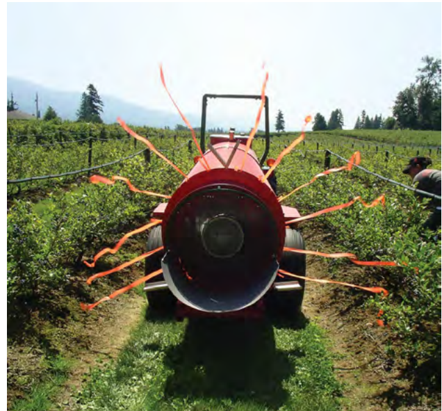
Figure 10. Using ribbons to work out where the air is being directed from the sprayer. Photo: Jason Deveau, Sprayers 101.
