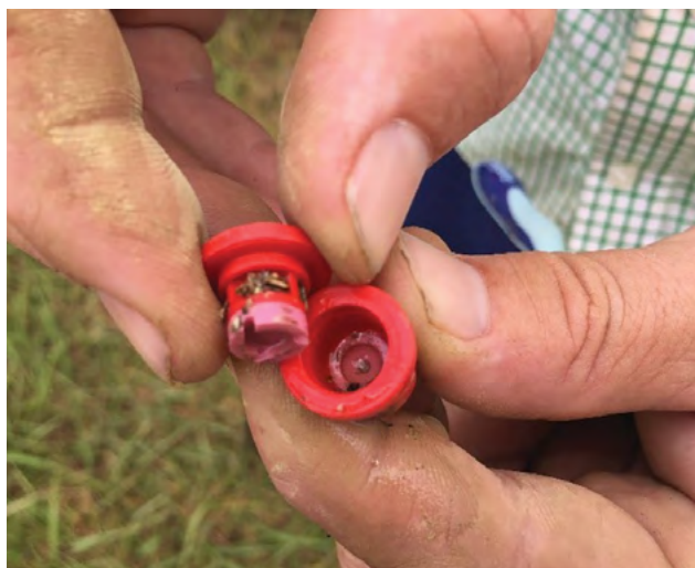
Figure 6. Nozzles should be cleaned regularly. Photo: Melinda Simpson.
